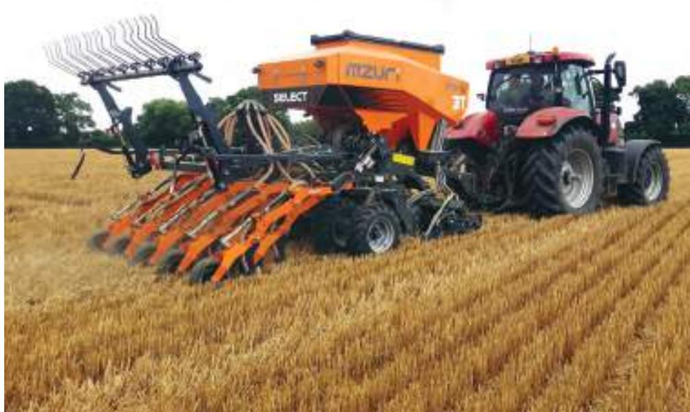
Strip tillage crop establishment with a three-metre trailed version of the Mzuri Pro-Til Select drill. (Photo: Mzuri)
