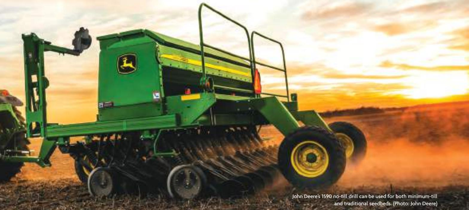
John Deere's 1590 no-till drill can be used for both minimum-till and traditional seedbeds. (Photo: John Deere)
